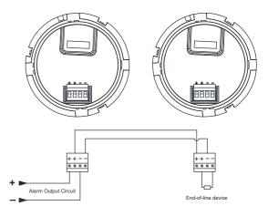
Fig. 2: Terminal loop wiring connections
