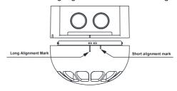
Fig. 3: Fitting the audio/visual alarm device to the backbox
