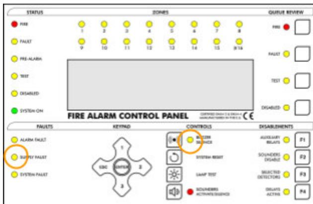
After a short delay, the SUPPLY FAULT LED will be ON, the panel buzzer sounds and the "Battery Fault" message appears on the LCD Display.
