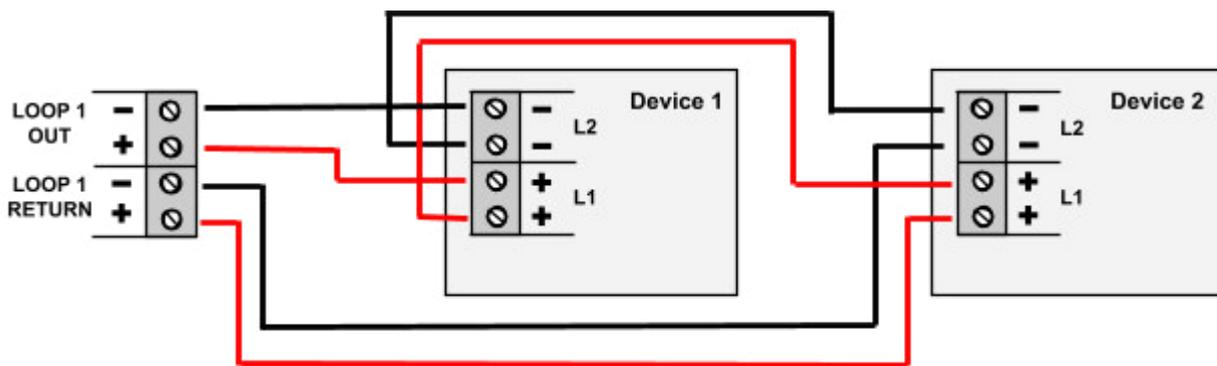
**NOTE:** A maximum of 32 manual call-points can be fitted into an Analogue loop. If this value is exceeded, the response time for certain types of call-points will be excessive.
