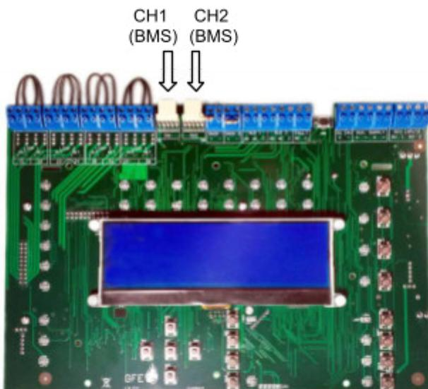
The GEKKO Panel may be incorporated into a Chameleon network. This also includes OCTO+, NODE+ or CHAMELEON REP. RS422, Fibre-Optic or TCP/IP connections may be used to connect them to a network.
