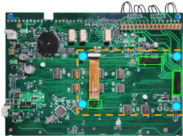
2 Male 20-way headers and 1 Male 8-way headers on expansion board should fit into the corresponding female headers situated at the back of the panel's main board.
