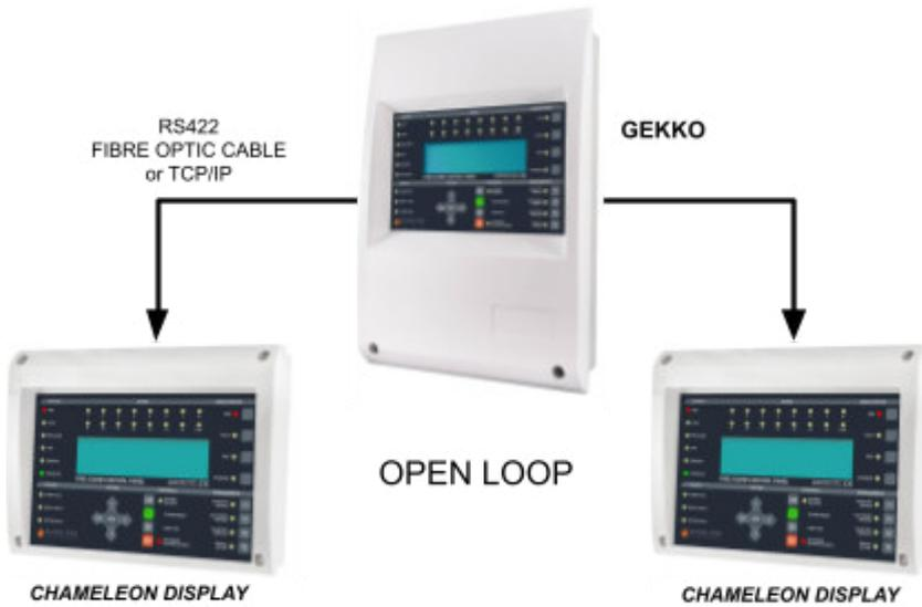
The Chameleon Display is commonly used when one or two simple display repeaters are needed on a “not networked” GEKKO.
