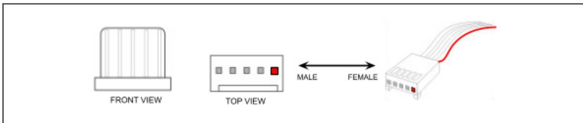
**NOTE:** Throughout the manual, the red pin on the 5 way molex indicates which pin is n°1.
