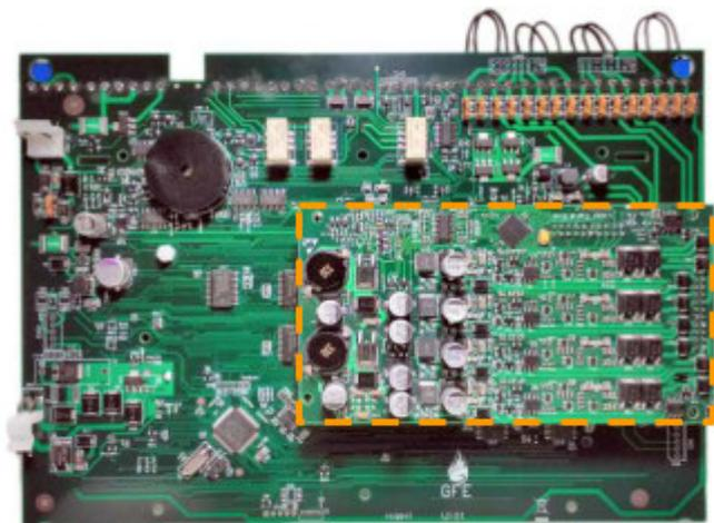
GEKKO Loop Card after fitting is completed.
