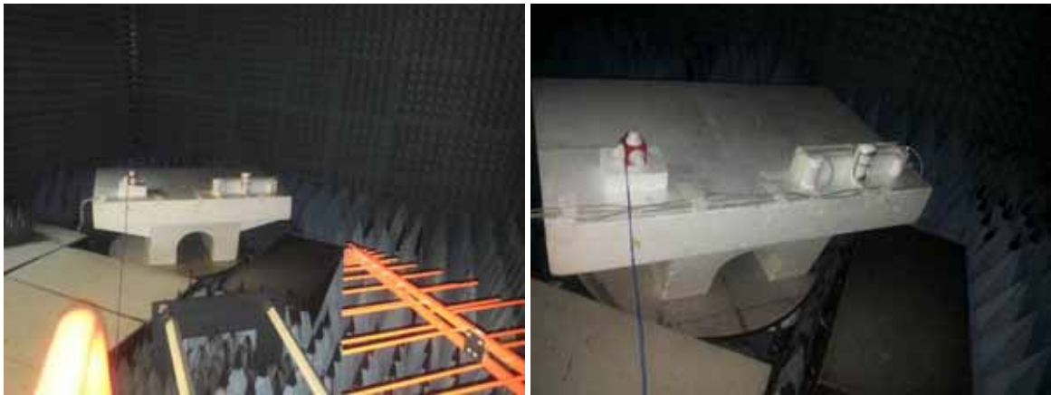
Photograph 7.1.6 Setup for radiated immunity to RF electromagnetic field test in 1000 – 2700 MHz range, DM70, DG85, NV5, PMD75 models
