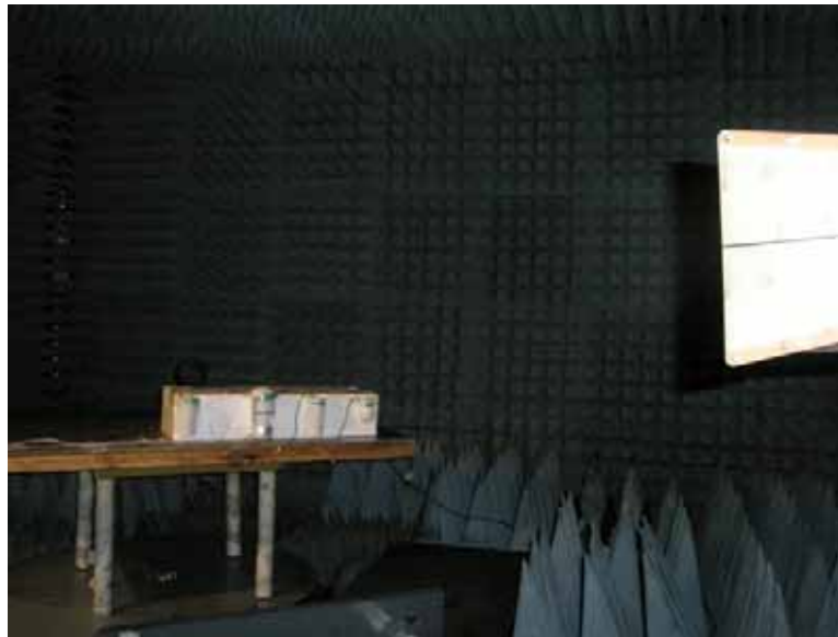
Photograph 7.1.6 Setup for radiated immunity to RF electromagnetic field test in 1000 – 2700 MHz range, DM70, DG85, NV5, PMD75 models
