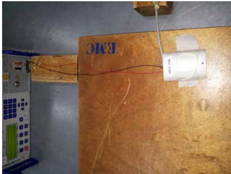
Photograph 7.2.6 Setup for conducted immunity to EFT/B at DC power supply line, 525DM model
