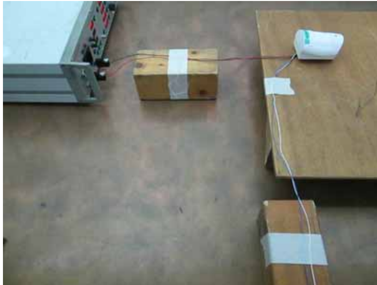
Photograph 7.2.2 Setup for conducted immunity to EFT/B at DC power supply line, DG55 model
