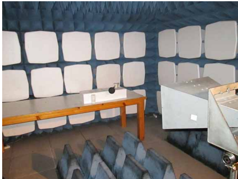
Photograph 7.1.2 Setup for radiated immunity to RF electromagnetic field test in 1000 – 2700 MHz range, PMD2P model
