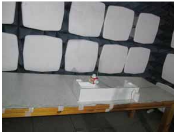
Photograph 7.1.11 Setup for radiated immunity to RF electromagnetic field test in 2000 – 2700 MHz range, DG55 model
