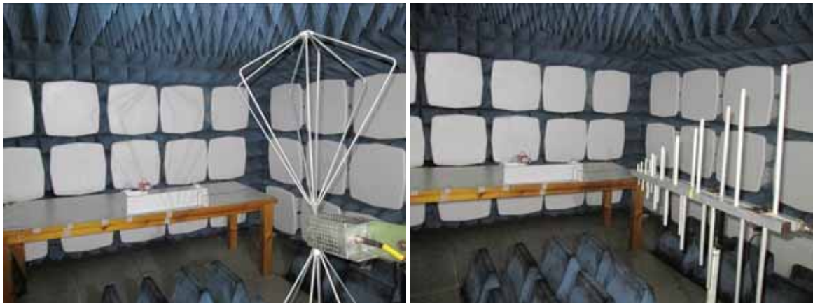
Photograph 7.1.10 Setup for radiated immunity to RF electromagnetic field test in 80 – 1000 MHz range, DG55 model
