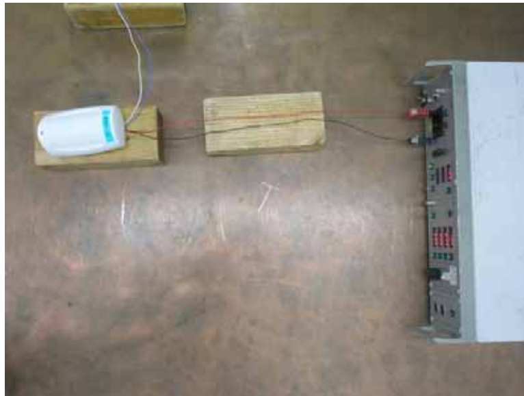
Photograph 7.2.4 Setup for conducted immunity to EFT/B at DC power supply line, DG65 model
