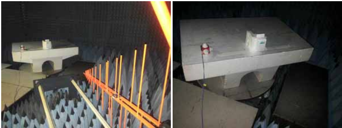
Photograph 7.1.4 Setup for radiated immunity to RF electromagnetic field test in 1000 – 2700 MHz range, NVR780 model
