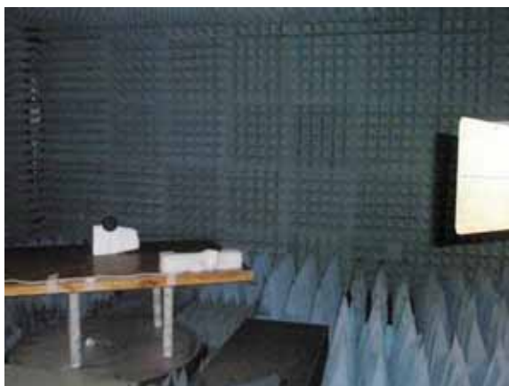
Photograph 7.1.11 Setup for radiated immunity to RF electromagnetic field test in 2000 – 2700 MHz range, DG55 model
