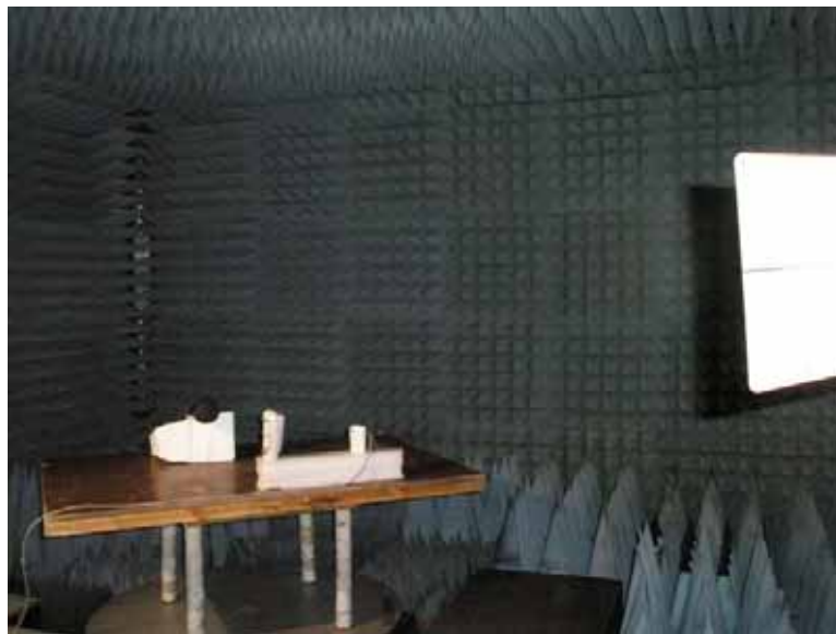
Photograph 7.1.7 Setup for radiated immunity to RF electromagnetic field test in 1000 – 2700 MHz range, DM50, PMD85 models
