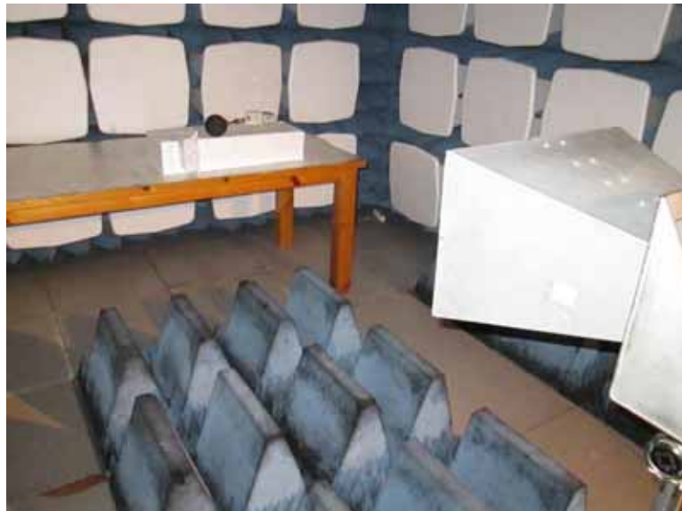
Photograph 7.1.4 Setup for radiated immunity to RF electromagnetic field test in 1000 – 2700 MHz range, NVR780 model
